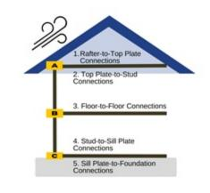
Homes with insufficient wind resistance can be made safer with continuous load path retrofits. These create a continuous connection between a house's roof and foundation to help keep the roof from blowing off during a hurricane. The goal of retrofitting is to add as many as reasonably possible, starting at the top (A1) and working down (C5).
